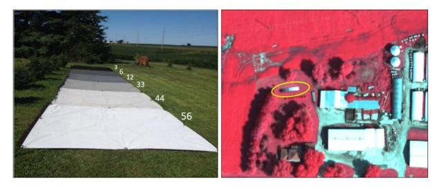
Figure 1. On-the-ground imagery calibration tarps with different percentage reflectance values (left). Tarps as seen in digital aerial imagery (right).
